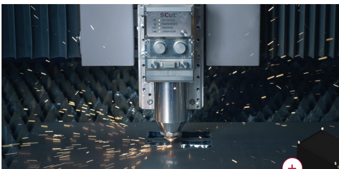
Bundle of SCut optics with laser and spliced 100 \mu\text{m} fiber
